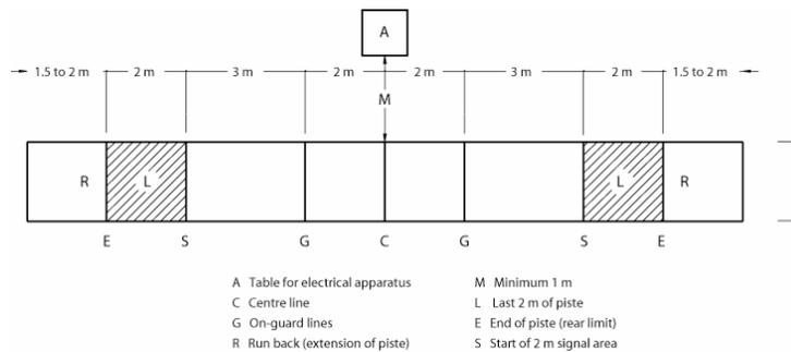
For foil and épée the conductive surface must cover the whole of the length and breadth of the piste, including its extensions (run back) (cf. Article L13s, m.57)
