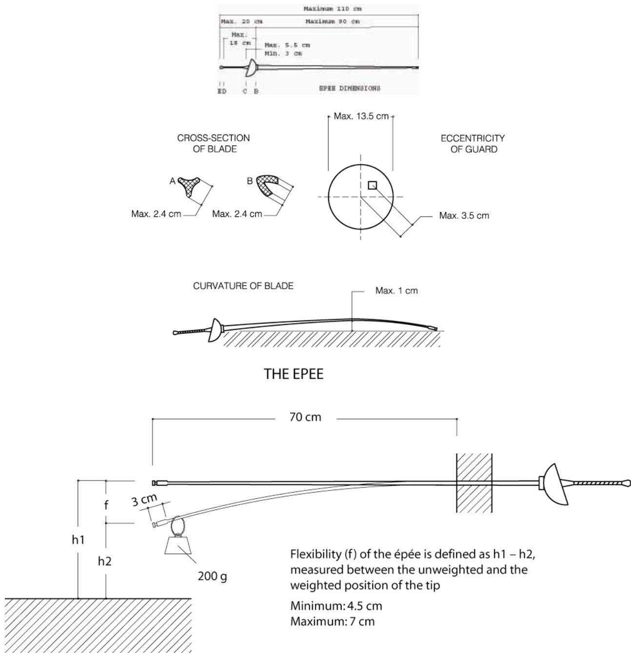
**Figure 9. Epee dimensions and flexibility**
