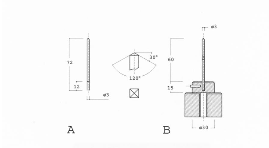
Figure A.4. High speed dynamometer for test of cloth resistance to perforation
