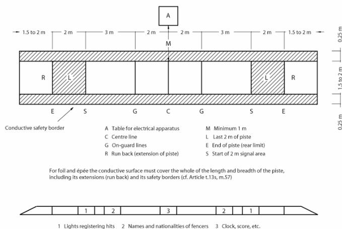
**Figure 1. Strip for Semi-Finals and Finals (maximum height 50 cm)**
