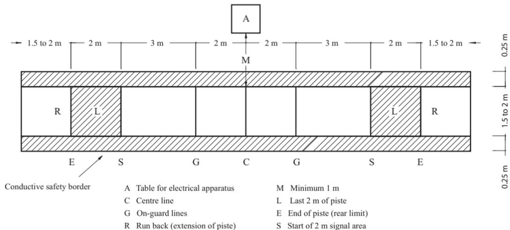
For foil and épée the conductive surface must cover the whole of the length and breadth of the piste, including its extensions (run back) and its safety borders (cf. Article t.13s, m.57)
