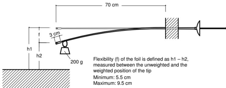
**Figure 8. Foil dimensions and flexibility**
